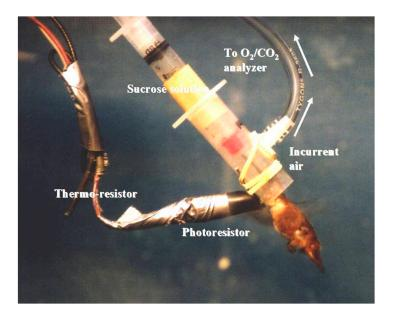
**Figure 2.** Hummingbird mask respirometry. The bird is freely hovering while feeding on a sucrose solution with its head in feeder modified to function as a mask for flow-through respirometry. Air is drawn into the mask at a known flow rate. The air, depleted of  $O_2$  and enriched with  $CO_2$ , is analyzed downstream using  $O_2$  and  $CO_2$  analyzers. See [20,26] for detailed description of the method.
